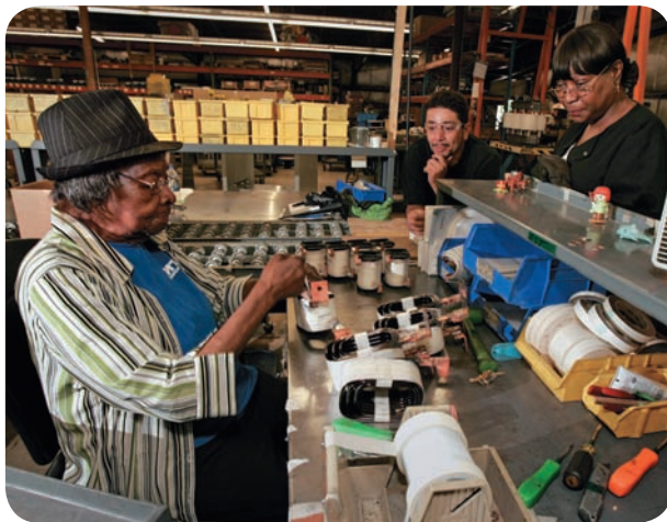
Ruby Johnson, 93, wraps heat-resistant tape around coils to insulate an electrical terminal at the company where she works in Menomonee Falls, Wisconsin. What are some variations in work and retirement in older adults?
